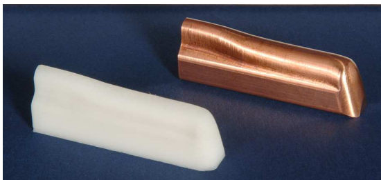
Figure 2: Final test piece (right), of the RFQ radial matcher section and a plastic model (left) to check the production procedures.
