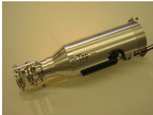
Figure 2: Plunger removed from the housing shown in Fig.1. At the left side frames and cones for stretching the target and degrader foils can be seen. The black cylinder is the housing of the piezo-motor including an optical device for measuring the target-degrader separation.
