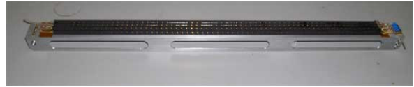
Figure 3: Straw tube prototypes: straw thickness 126 \mu m; capton on Al (0.2 \mu m) covered by C-layer (5 \mu m). Length = 60 cm; Inner diameter = 7.5 mm. Ar/CO 2 (80/20) at atmospheric pressure at 1850 V.
