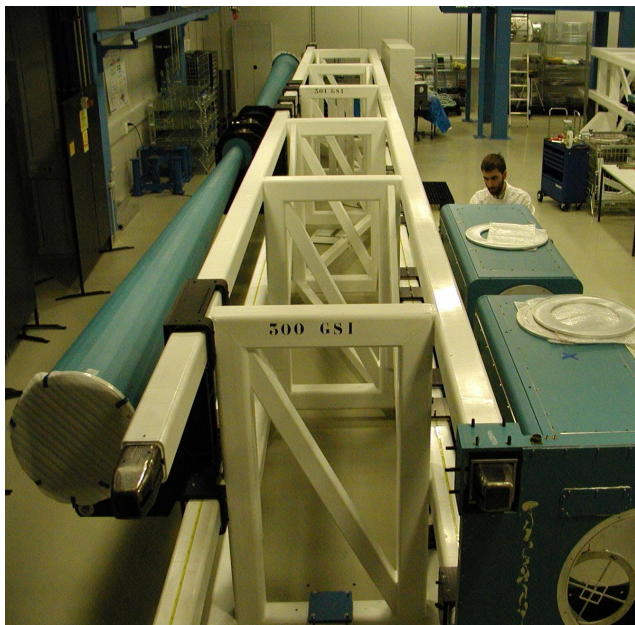
Fig. 3: Mechanical adaptation of the laser components for the main amplifier chain has proceeded. On the right hand side, amplifier modules are mounted. On the left hand side, the spatial filter telescope is modified for the 2-pass design.
