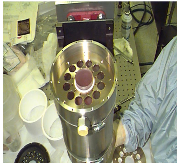
Fig. 2 : The 45 mm amplifier of the pre-amplifier section. The Nd:Glass amplifier rod is surrounded by 12 flash lamps.
