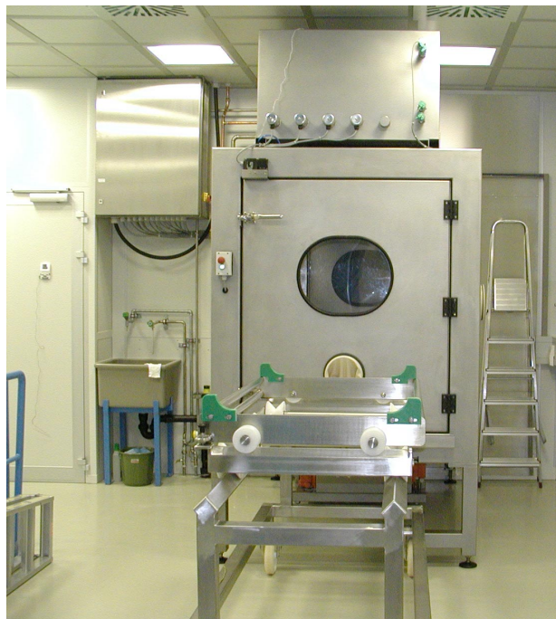
Fig. 4: The high pressure water spray booth for the cleaning of the amplifier housings operates with de-ionized water to avoid residues on the optics, at temperatures up to 60C. It also serves as lock-gate for components being introduced into the class-100 clean room facility located at the other side of the wall.
