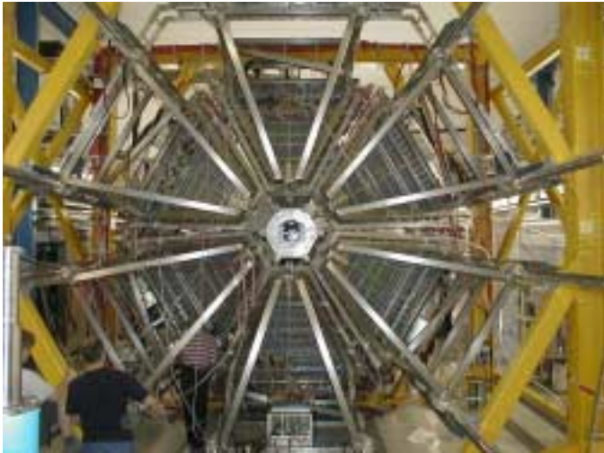
Figure 1: Upstream view of the Hades setup. Only the support structure and outermost detector layer (Pre-Shower detector, part of TOF) are visible.
