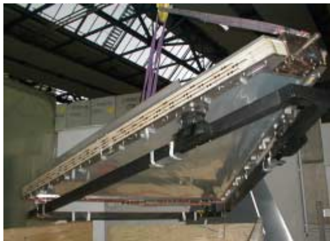
Figure 4: Picture showing the first plane IV module arriving at GSI. For transportation the chamber is mounted on a support structure via surge dampers. It has a height of 3 m and weighs about 200 kg.
