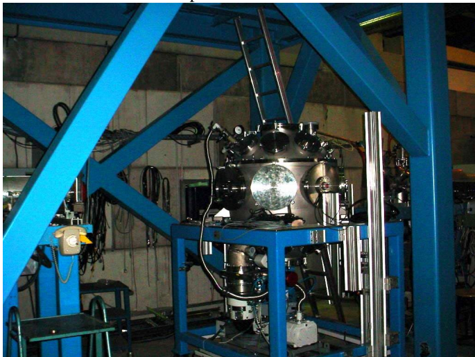
Fig. 5: Shown is the new target chamber at Z6 below the last mirror tower. The ion beam from the UNILAC arrives from the right hand side, while the laser pulse arrives either from the top or from the top left.
