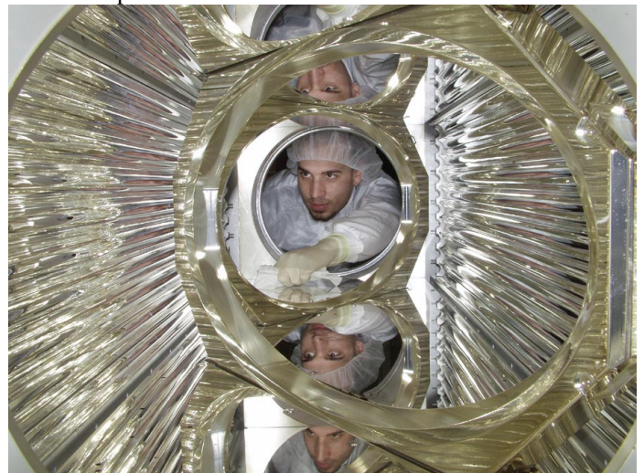
Figure 2.: PHELIX engineers clean an A315 amplifiers in preparation for the usage. Shown is the inside of the amplifier with two laser disk holders in the middle and flashlamp panels on the left and right. (Picture: G. Otto)
