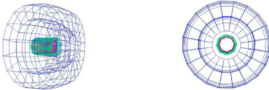
Figure 2. General scheme of the recoil detector. The red cylinder represents the first layer and the green cylinder the second layer of the tracker. The calorimeter is indicated in blue.
