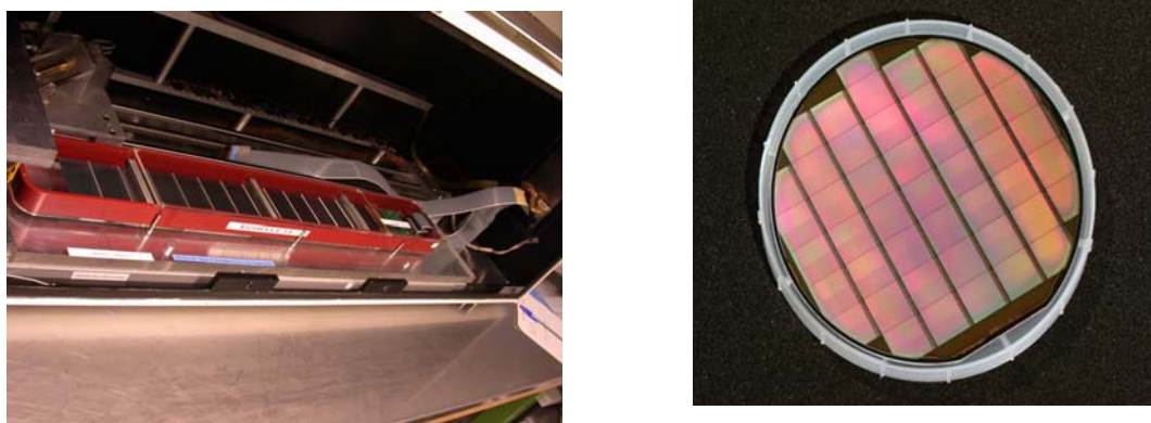
Figure 6. Left: Example of the arrangement of the double-sided Si detectors on a ladder (a part of the tracker system of the AMS experiment). Right: Prototypes of the MAPS detectors on 6" Si wafer.
