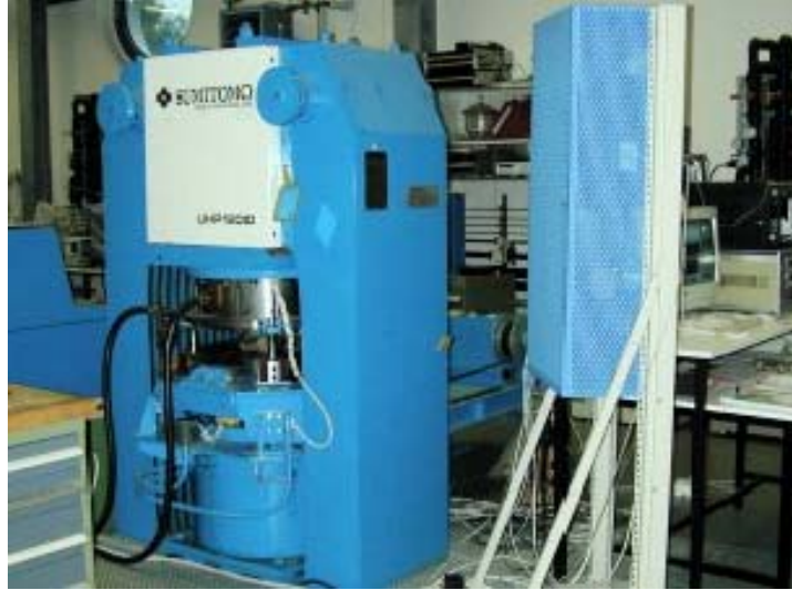
Fig. 9: Ultrahigh-pressure facility with large-volume multi-anvil cell (taken from the homepage of Bayerisches Geoinstitut, Bayerische Akademie der Wissenschaften, Bayreuth).
