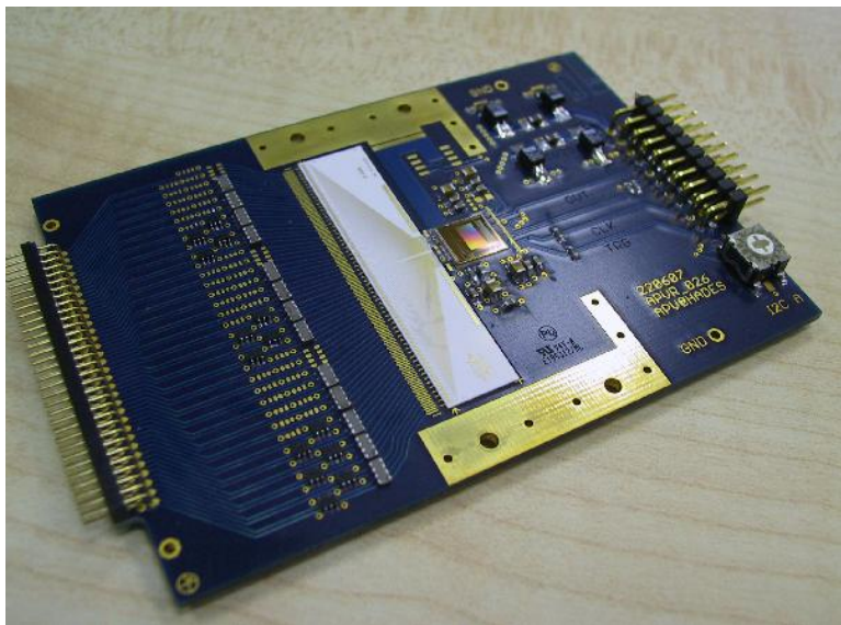
Figure 5: New APV-front-end board for 128 channels (left); GTB bridge board with 4 ADCs to connect 4 of the front-end boards to the digital GTB bus (right).
