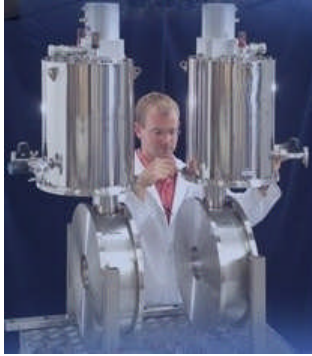
Figure 1.2.a : Photo of the two HTS Coils Cryostats built at Culham.
