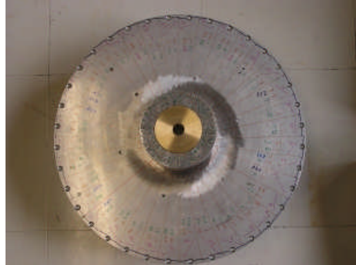
Figure 1.5.b : lateral hexapole fitted with permanent magnets
