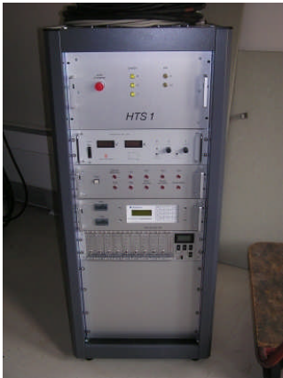
Figure 7.a : Quench detection electronic for HTS Coil 1
