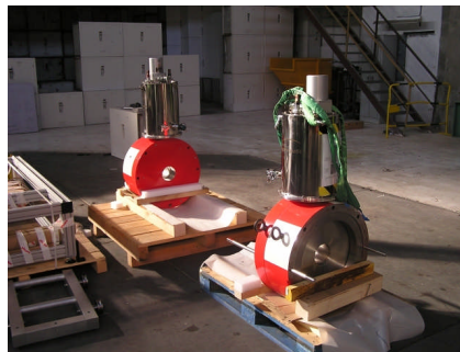
Figure 2.3: HTS Coils in their cryostats, surrounded with their iron yoke.
