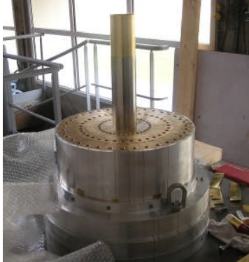
Figure 1.5.a : Centre hexapole cylinder which will contain the permanent magnets. At this stage, it is filled with brass mechanical parts that will help for final magnet assembly.
