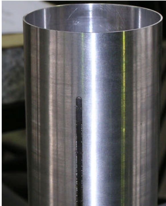
Figure 3.5 : successful laser welding of the iron plate in the body of the plasma chamber
