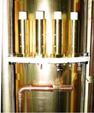
Figure 12: Resonance circuit and glass probe at the analysing plane region. The resonance circuit is an LC circuit that matches to the impedance of the sending-receiving electronics. To fulfil the extreme requirements of UH vacuum and low temperatures the LC components have been designed in vacuum-compatible materials with very similar dilatation coefficients.
