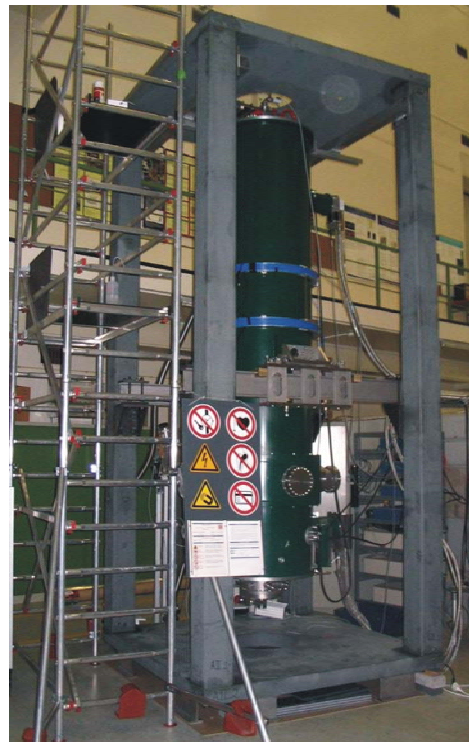
Figure 6: Left: The magnetic field in the symmetry plane that cuts through a pillar of the anti-magnetic screen. Right: Setup of aSPECT inside the shield, a combination of construction steel (plates of cross-section 180x180cm 2 and thickness 10cm) and ARMCO iron (pillars of cross-section 20x20cm 2 and length 400cm).
